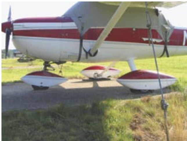
Three flat tires are the first sure sign of a neglected aircraft.
